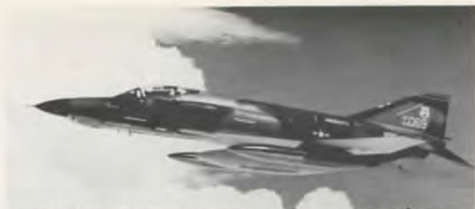
The Duluth-based 148th Tactical Reconnaissance Group's new aircraft — the RF-4 "Phantom" Aerial Reconnaissance Aircraft, capable of low-altitude, high speed recon missions using cameras, radar and sensors
