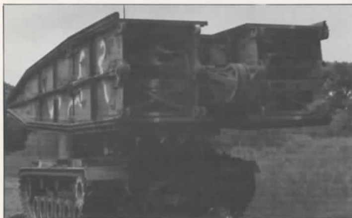
The new mobile bridge launcher, capable of bridging 60-foot ravines and streams
