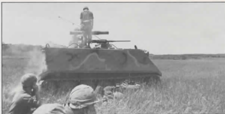
TOW gunner optically tracks the missile into the target
