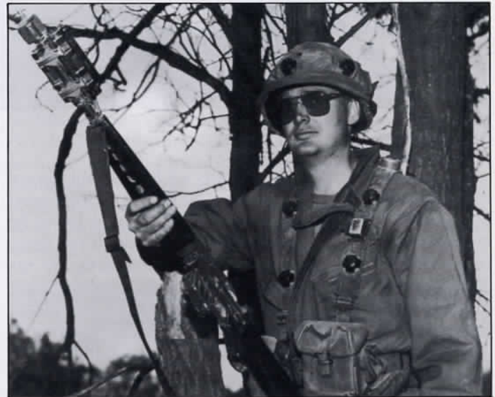
MILES equipment transmits and senses harmless laser beams simulating battle casualties and enhances realism
