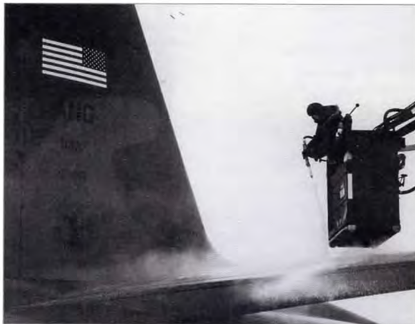
A Minnesota Air National Guard C-130 Hercules is de-iced prior to take-off.
